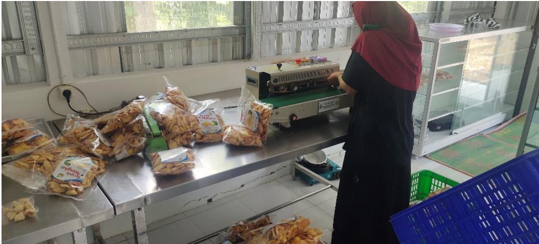
Gambar 16. Proses sealer kemasan keripik
