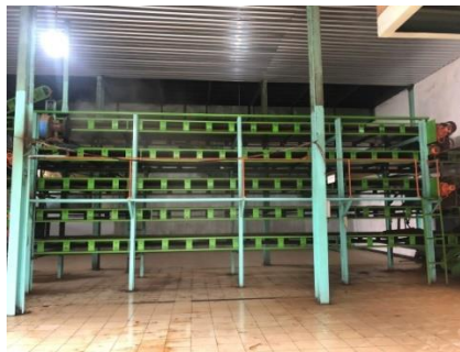
Gambar 4.20 Continuous Fermenting Unit
