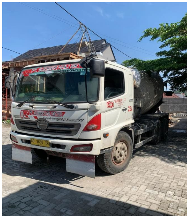
(Gambar 4.6 Truk molen beton readymix K-225)
