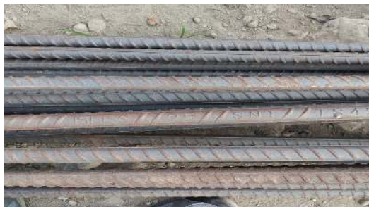
Gambar 4.2 Besi tulangan ulir (sirip) diameter 25 mm
